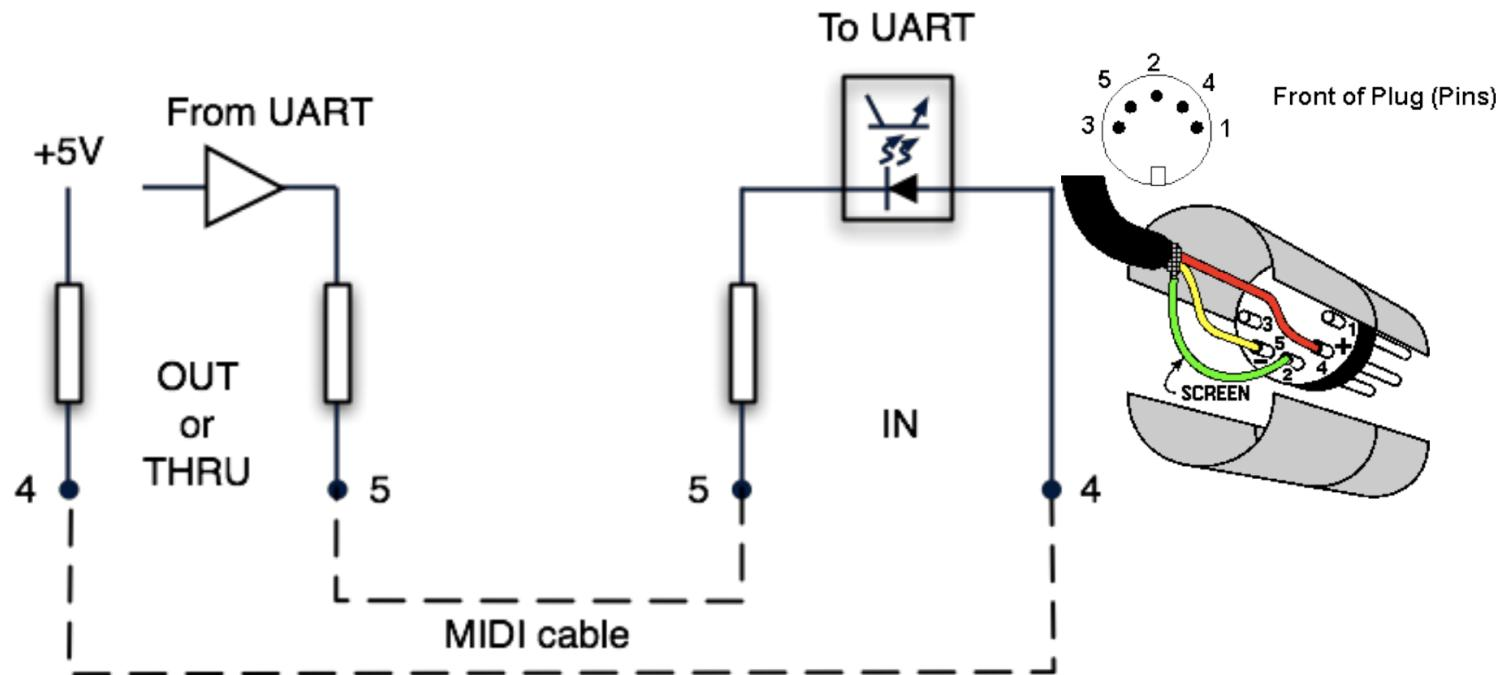
\* **UART** stands for "Universal Asynchronous Receiver/Transmitter". It is a piece of digital hardware that transports bytes between digital devices, commonly found as a peripheral on computer and microcontroller systems. It is the device that underlies a serial port, and it is also used by **MIDI**.
